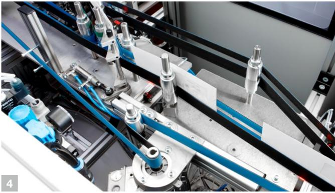
4 New secure envelope transport for high cycle speeds. Easy to maintain with good visibility for the operator.
