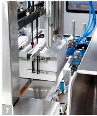
7 Compact filling station with diverter, the PBSplus High Performance comes with a second filling station in tandem operation for small groups at high speed.
