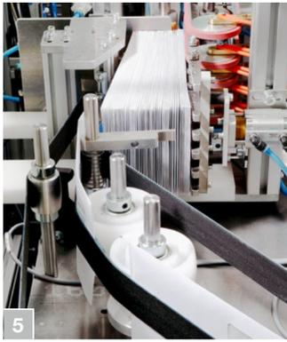
5 Integrated buffer and short tray exchange times, reduce the number of reprints. Impact on the inserter cycle speed is reduced to a minimum.
